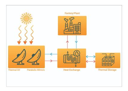
Infographic: Concentrated Solar Thermal (CST) platform and Thermal Storage unit together with BoP ("heat exchange") at Avery Dennison factory.
